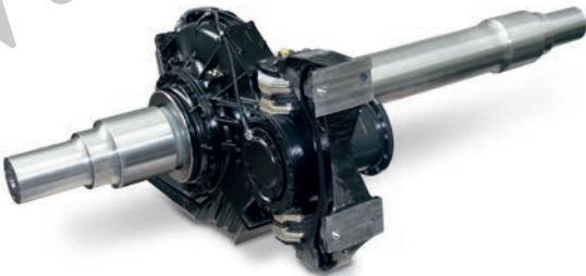
Wheelset transmission with aluminum housing for modern high-speed trains
